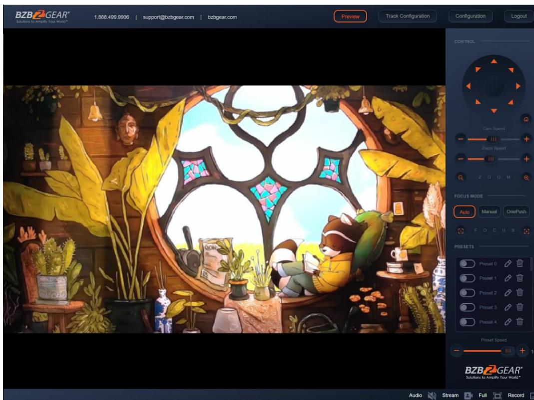
After successfully logging into the management interface, the web portal will enter the “Preview” tab. In Preview, users can control pan/tilt, zoom, focus, video capture, sound, focus, full screen preview, as well as set the preset position, run, delete, and other operations.
