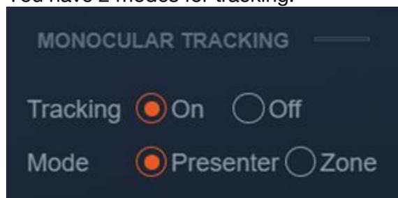
**Presenter:** The camera will continuously follow the subject until either the subject moves beyond the camera’s physical range of motion, a new more prominent target is in frame, or the tracking is disabled. The Adamo can accurately track subjects up to 6-7 meters away walking at speeds of up to 5-6 mph.
